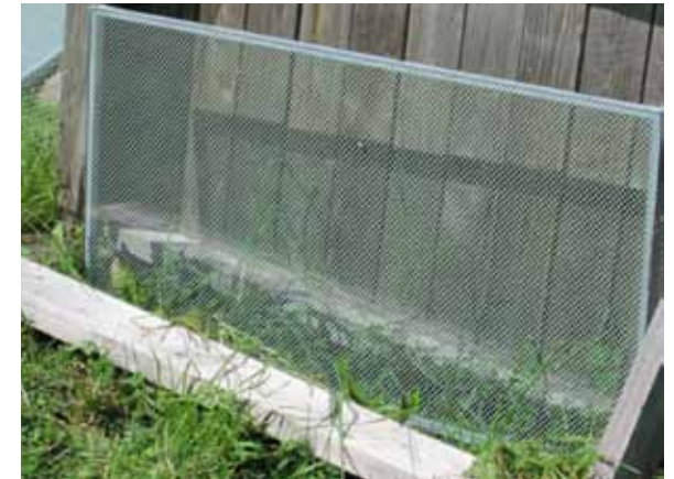
All-over patterns such as the one shown above are less effective at deterring collisions. Patterns with more contrast and distinct spaces, such as the one shown on the left, are much more effective. Photo: Christine Sheppard, ABC
