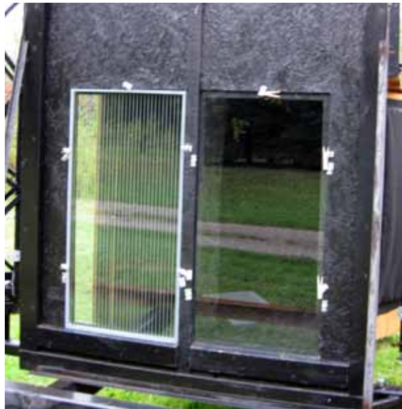
A panel of fritted glass, ready for testing. Photo: Christine Sheppard, ABC
