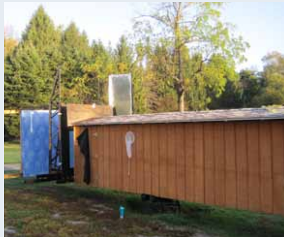
The tunnel – an apparatus for safely testing effectiveness of different materials and designs for deterring bird collisions. Photo: Christine Sheppard, ABC
